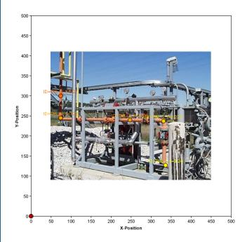
Data point IDs, thickness and MAWP are shown indicating areas of material loss. Color codes are user configurable for indicating high to low areas of material loss.
