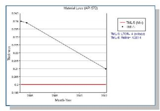
Provides MAWP and end of life calculation based on input parameters of tube diameter, yield stress, metal temperature and measured thickness. MAWP comparison with operating pressure assists in determining continued operating risk.
