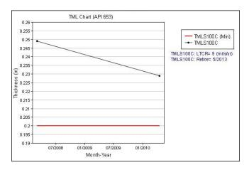
MI Manager provides MAWP and end of life calculation based on input parameters of component diameter, yield stress, metal temperature and measured thickness. MAWP comparison with operating pressure assists in determining continued operating risk.
