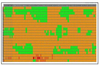
Tank floor and roof data points are shown as color coded points. Points that color red indicate areas of concern.
