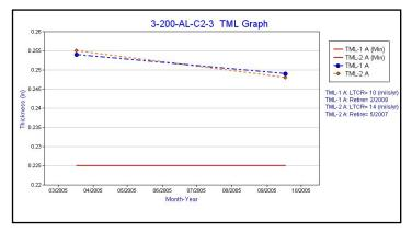
Inspections that involve thicknesses can be graphed and viewed for trends. TML graph provides LTCR calculation and projected asset retire date based on TML(s) selected. Analyze corrosion rates for piping circuits, storage tanks and pressure vessels.
